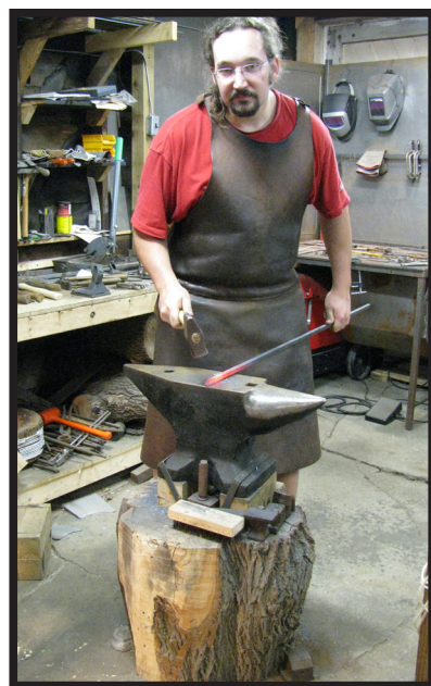
Chip in a leather apron of his own design hammering hot iron on an Italian pattern double-horned anvil.
