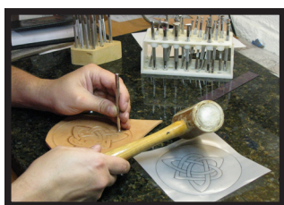
Aligning the beveler to add further definition
