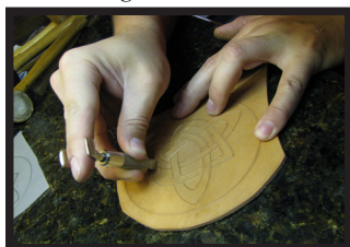
Carving out the pattern with a swivel knife
