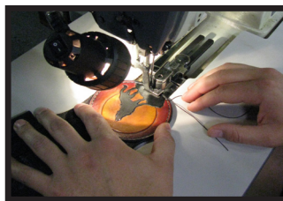
Sewing station: sewing the decorative detail onto the pouch
